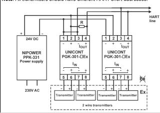
R = 300 Ohm / 2W...1 kOhm / 2 W should be between these values depending on the number of the applied isolator modules. It should be connected to only one unit! Resistance value of the necessary resistor can be calculated by the help of the following formula:
