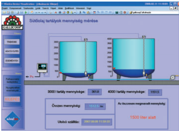
Level measurement in oil tanks: With MicroTREK , MULTICONT instruments, data logging, trend monitoring and database handling.
